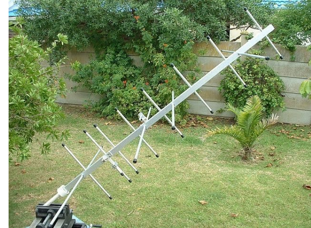
High Gain Yagi >20dB
